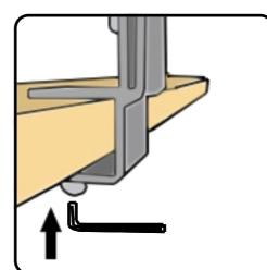
2. Tighten Screws at base of eachclamp. Do NOT over tighten or damage will occur.
