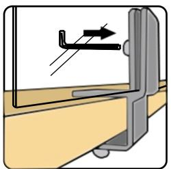
4. Tighten Screws at top of each clamp. Do NOT over tighten or damage will occur.
